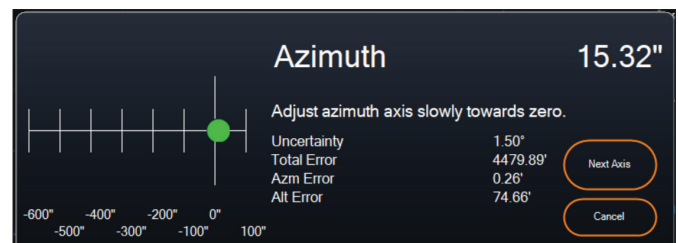
Fig. 18: Azimuth Axis Adjustment window during polar alignment in CPWI.
